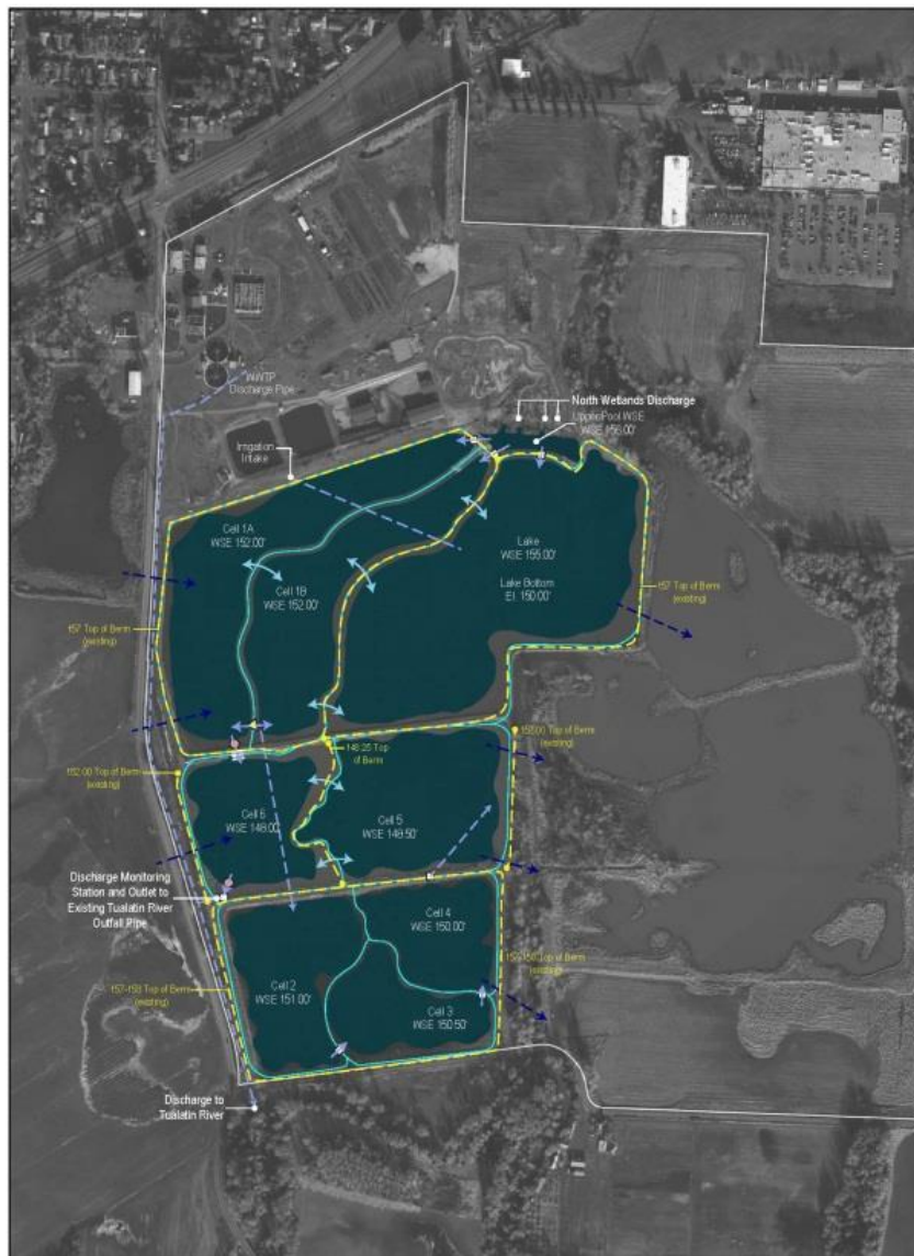
Figure 5-1 Basis of Design Normal Operating Water Level
