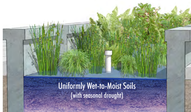
Planting conditions for LIDA facilities without sloped edges (such as concrete flow-through planters and infiltration planters) are largely uniform.
